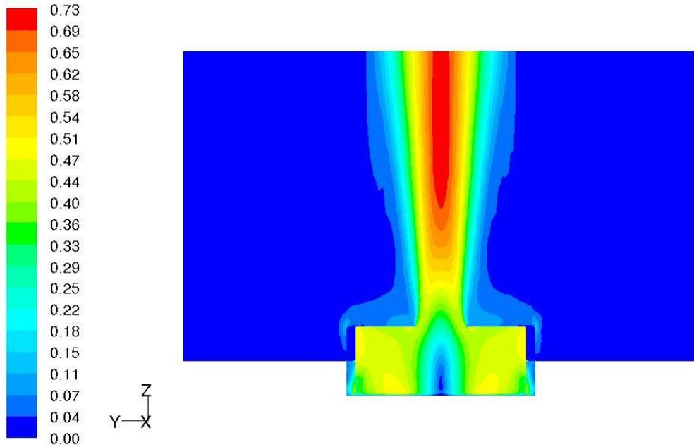
Figure 5.14: The contour plot of velocity magnitude (m/s) in the YZ plane for model-scale AVE with increased temperature difference between the inlet air and ambient air ( $\Delta T = 30$  K) (Turbulent Simulations)
