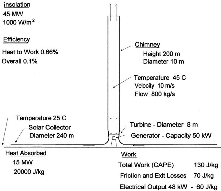
Fig. 1. Manzanares solar-chimney.
