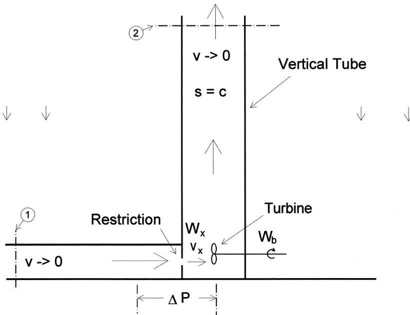
Fig. 3. Vertical tube with turbine at its base.
