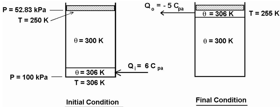
Fig. 2 Reversible process consisting of a column of dry air with uniform potential temperature. The heat that needs to be removed to restore the initial condition is less than the heat supplied because some of the heat is converted to work.
