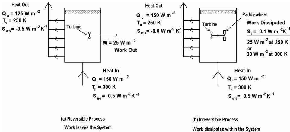
**Fig. 1** In reversible process (a) the heat out is less than the heat in because work is ignored, which is equivalent to letting the work leave the system. In irreversible process (b) the heat out is equal to the heat in because the work is dissipated within the system.
