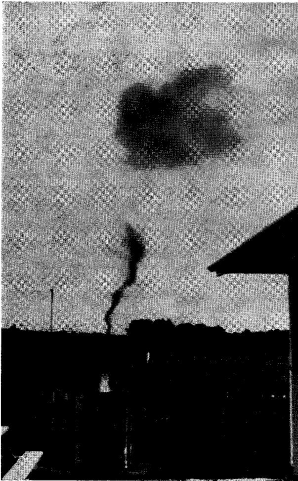
FIG. 2. Vortex produced by burning fuel inside a circle of deflectors.
